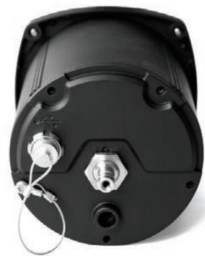
There are two variants of the i2O Remote Logger. The basic Remote Logger is fitted with a single pressure transducer only. The advanced Remote Logger has a smart expansion port which enables the logger to be upgraded to support additional external transducers, external batteries and external power sources.
